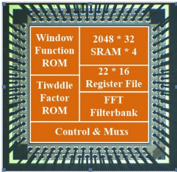
圖 9 Silicon implementation and gate count distribution
