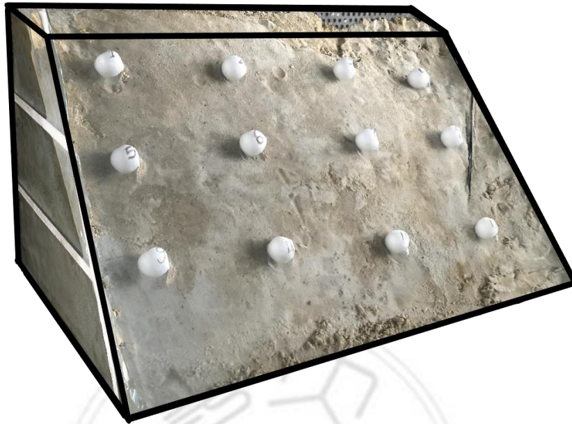
Figure 4-4: Cross section of the sample with foam balls to capture the movement of landslide
