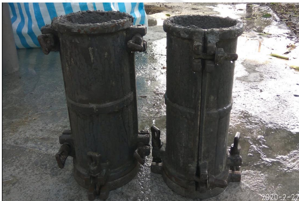
Figure 3. 5 Standard compressive strength cylinder mold
