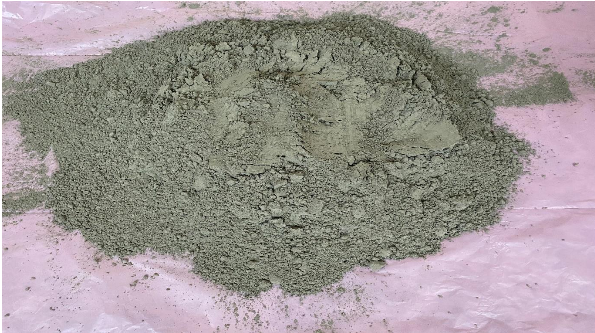
Figure 3. 1 Ordinary Portland cement
