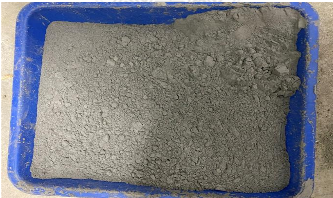
Figure 3. 4 Fly ash used as cement replacement
