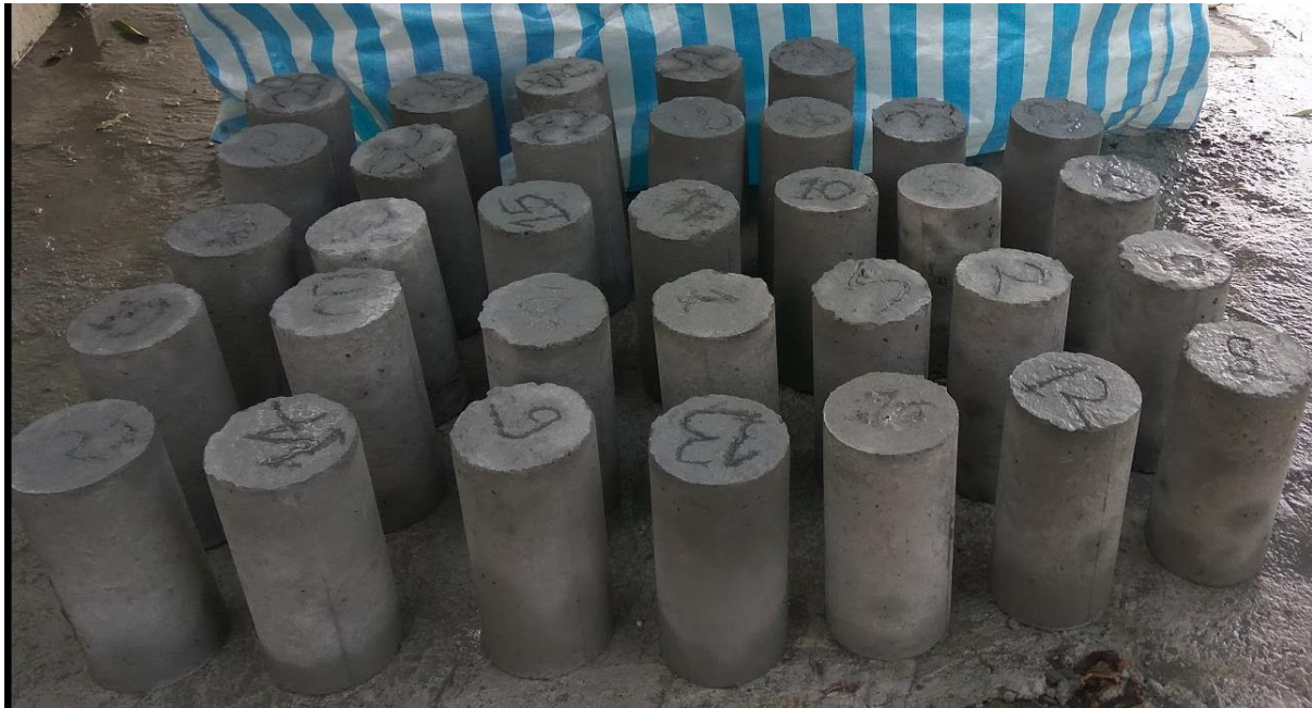
Figure 3. 10 Cylinder tested for compressive strength
