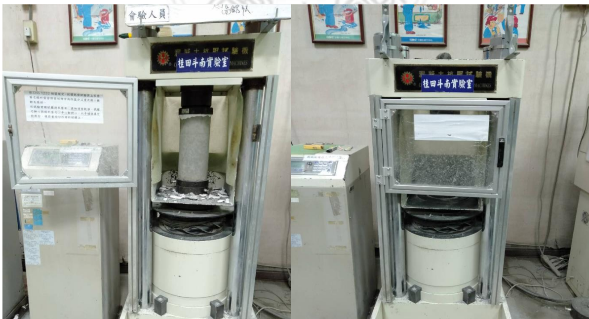
Figure 3. 11 Compressive strength testing machine with sample
