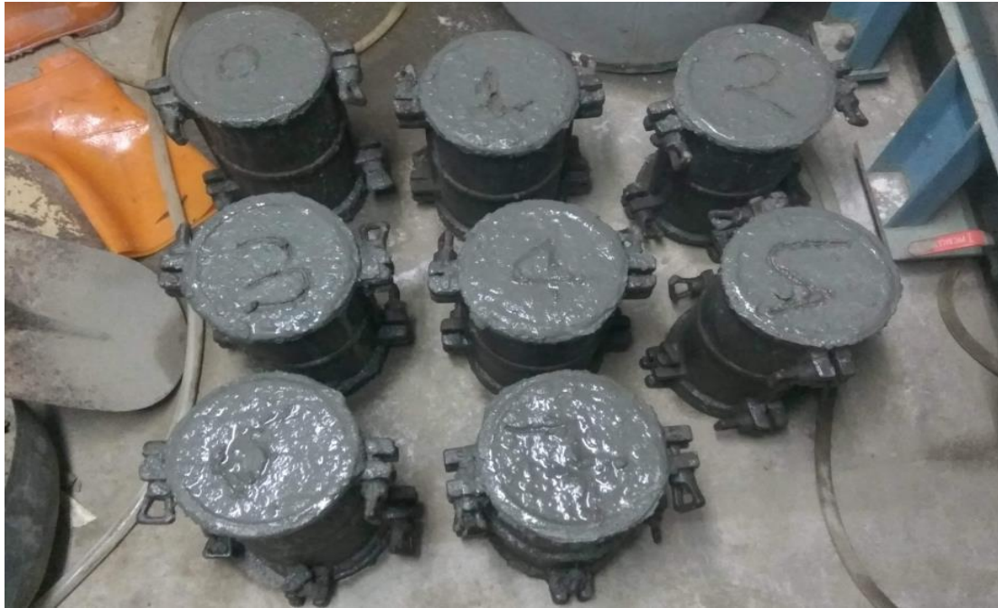
Figure 3. 9 Cylinder mold with a smooth surface
