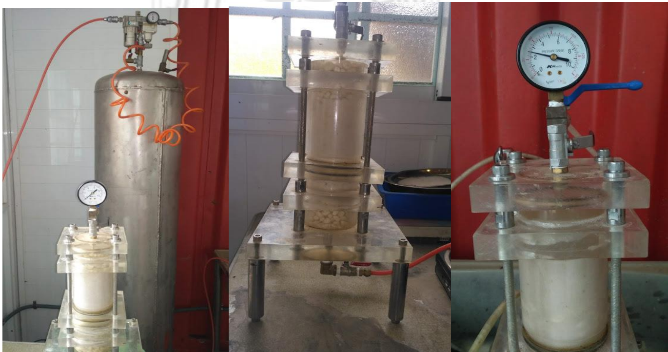
(a) Experimental setup for NEFT (b) Designed sample (c) Pressure
