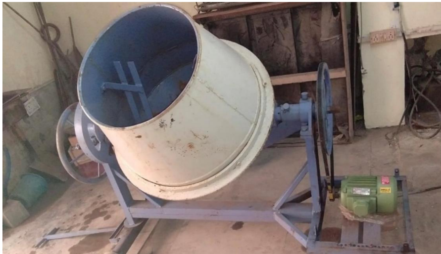
Figure 3.5: Concrete Mixture Machine
