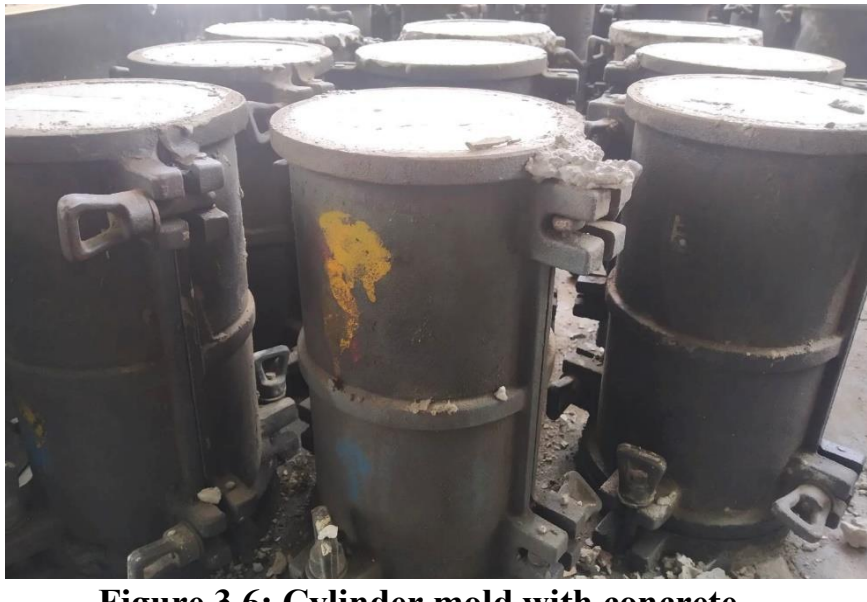
Figure 3.6: Cylinder mold with concrete
