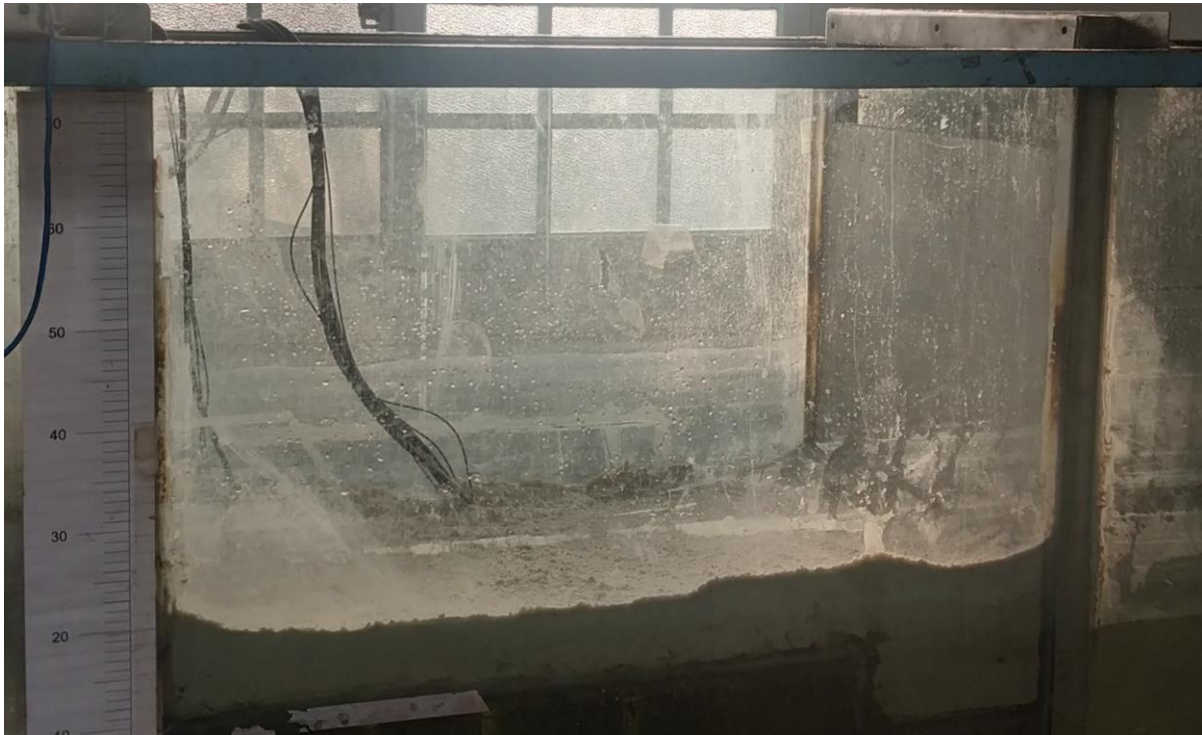
Figure 3-13: Setup for sensor calibration when subjected to water and soil both
