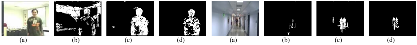
Fig. 3. Detection results of the first sequence: (a) original image, (b) Stauffer and Grimson's method, (c) Heikkilä and Pietikäinen's method, and (d) proposed method.
