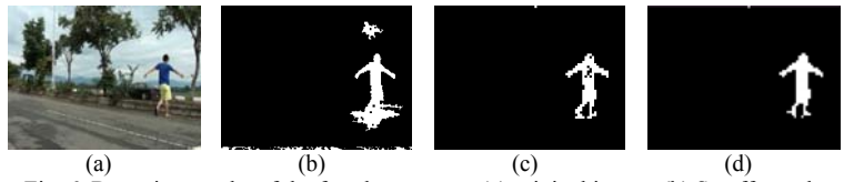
Fig. 6. Detection results of the fourth sequence: (a) original image, (b) Stauffer and Grimson's method, (c) proposed method, and (d) proposed method with morphology.
