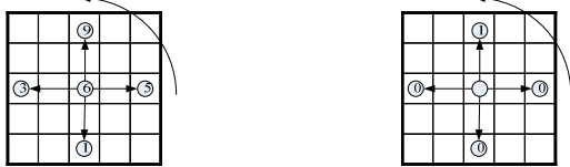
(a) Neighbors of the central pixel (b) Binary pattern Fig. 1. An example of generating LBP.
